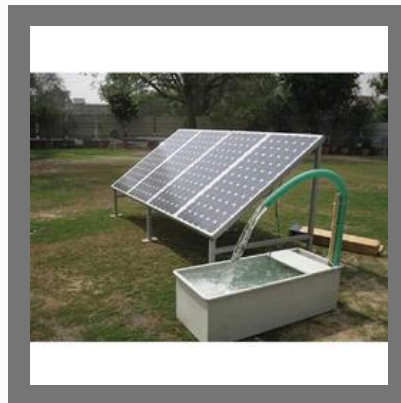
Solar Water Pumping System
